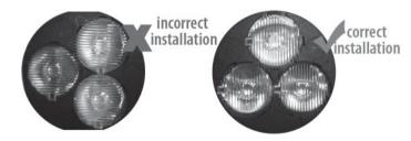
\*\*Annexe A: These wide angle lights must be correctly positioned. Look through the outer lens and you will see lines on the primary optics ie the 3 small lenses. The lines in the optic must be vertical, see photos\*\*
